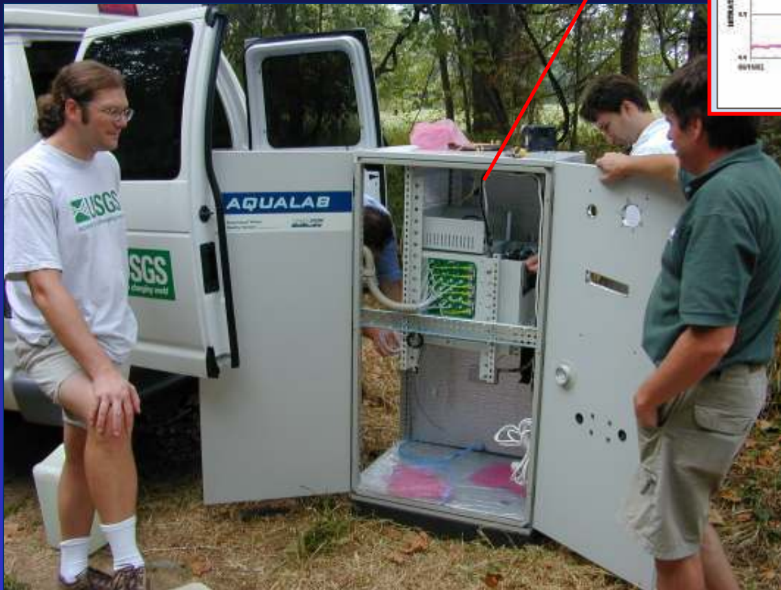
USGS Scientists preparing to install the Greenspan (now Stevens) AQUALAB Analyzer at Morgan Creek, Maryland. [Photo by James R. Jeffries, U.S. Geological Survey]
