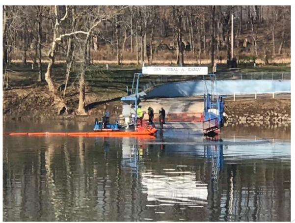
Ferry at VA side of river; unable to get boom to VA anchor point. Weight of ferry and water against boom caused concern for ferry cable break.
